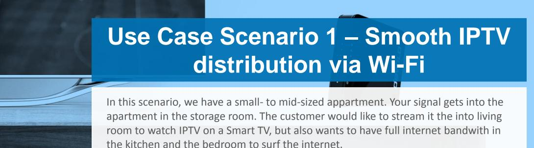
By connecting an OS WiFi Bridge Access Point to the gateway/router in the storage room, and placing it in the hallway, the IPTV signal will be transferred smoothly and reliably via a 5 GHz Wi-Fi network to the Smart TV. By adding an OS WiFi Bridge Station into the kitchen, the internet signal will be repeated by the Access
