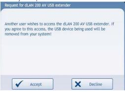
• If the other user accepts your request, you will automatically be connected with the dLAN 200 AV USB extender. The green USB symbol in the top left-hand corner of the dLAN 200 AV USB extender signals the now existing connection to the USB device.
