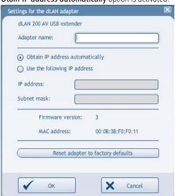
If a DHCP server is already available in the network for assignment of IP addresses (e.g. a PC), you should leave the **Obtain IP addresse automatically** option activated so that the dLAN 200 AV USB extender automatically receives and is found an address by this server.
